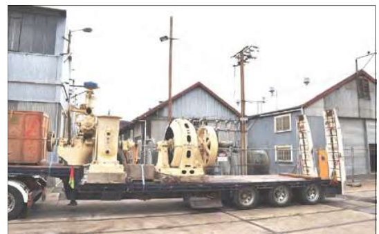
The turbine, generator and governor on the truck are the 445hp/300kW machine being transported from the Queen Victoria Museum bulk store to the workshop for disassembly, clean up and painting. Photo source not provided.
