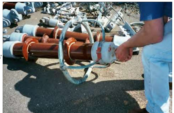
Insulators with corona rings.
