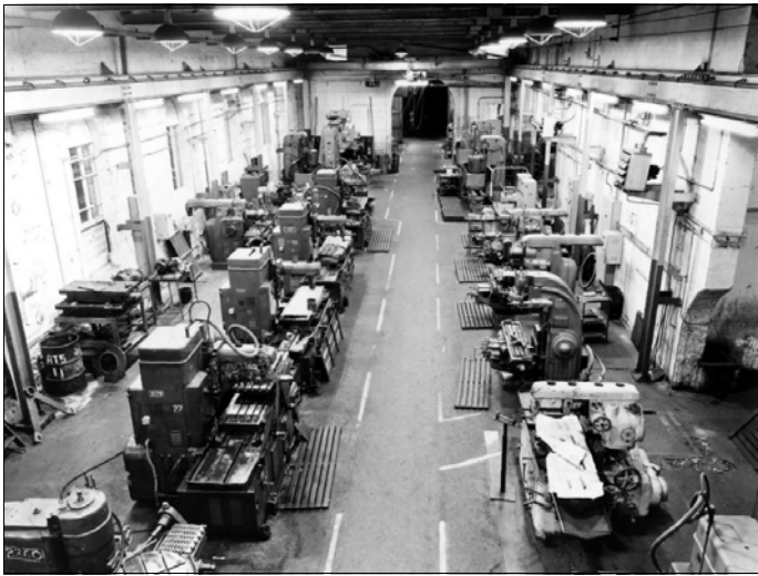
In preparation for the manufacture of steam turbines for the Daring-class destroyers and the Type 12 frigates, new milling machinery was installed in the machine shops (c1946). Contrast this tidy space with electric motor driven machinery replacing the line-shafting seen in a 1914 photo of the same space (see photo on a previous page). Source: J Jeremy collection.
