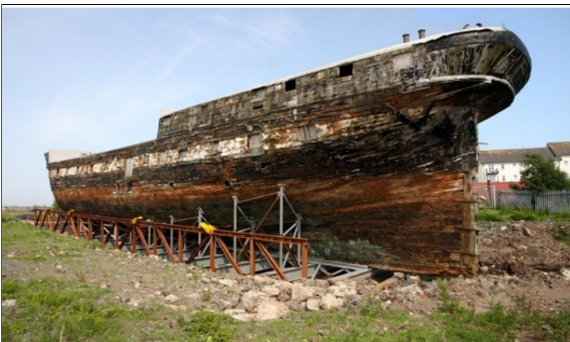
The shipping cradle reassembled under the Adelaide's hull in July 2013.
